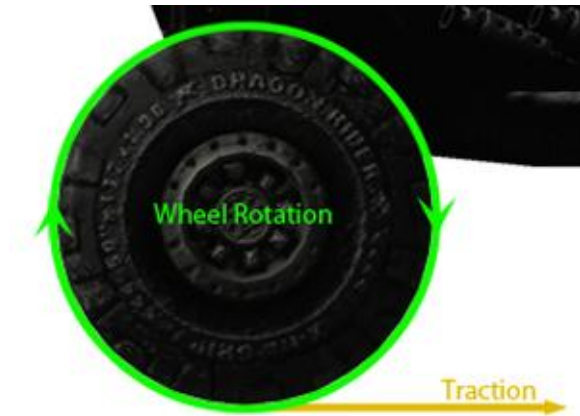
Figure 6: Driving wheel exerts the traction force on the road
